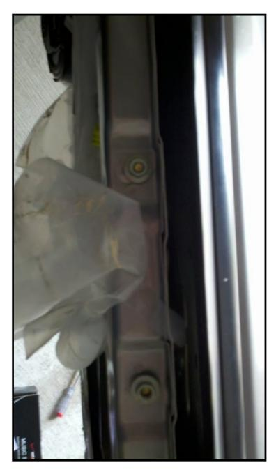
Using the 1/2" wrench, remove the bottom nuts.
