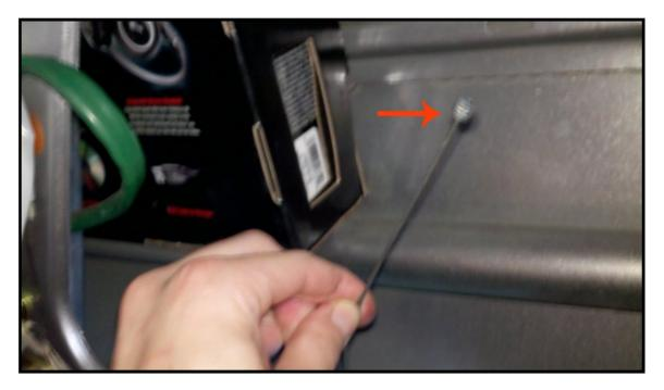
Step 3: Push the window upward from the bottom (you can then pull it out the top once it gets up halfway). It is best to have someone help hold the window up for you or you can try using heavy duty tape to hold it up. Or you can do what I do and hold it with one hand, try to do stuff with the other hand, and curse with the mouth.
