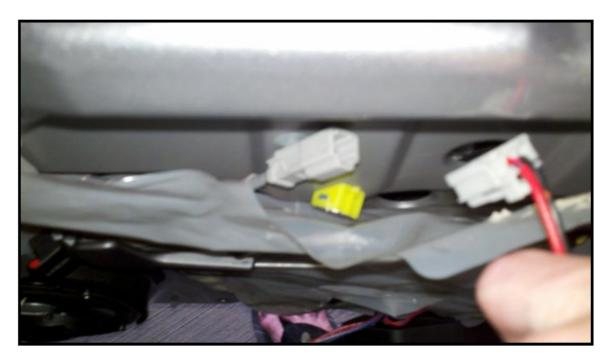
Then, follow all the steps in reverse order that you used to take off the door panel. Remember, there are two screws in the "oh shit" handle, one behind the door latch, and a clip style tab towards the front of the door panel.
