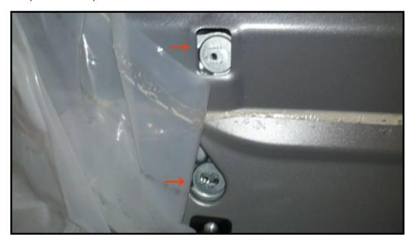
Next, you need to put the two little white plastic pieces back on. What you are looking to do is to get the upward angle of the non-round square piece to go in between where I marked with an arrow:
