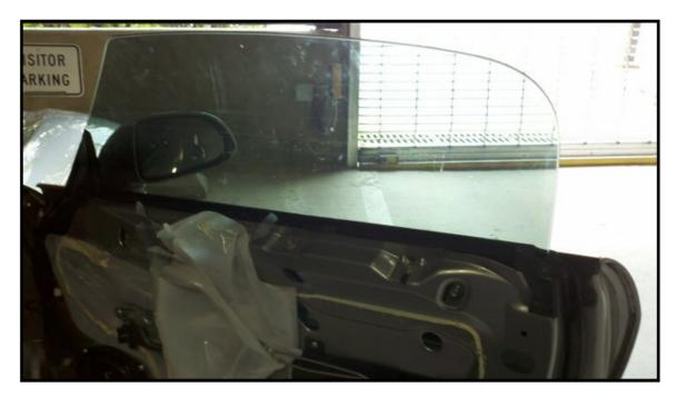
Then it is just a matter of putting the three nuts that hold on the glass back in. Remember, there are three of them (here are two):
